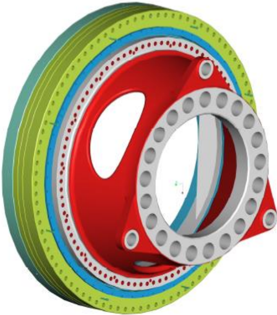
Figure 1 Dreireihiges Rotorlager / Three rowed Main Bearing
